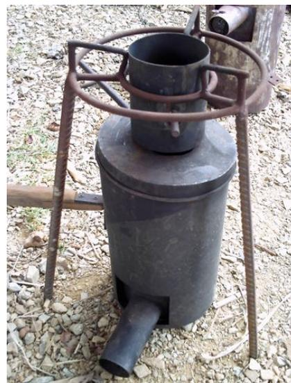
Examples of biochar-producing apparatus.
