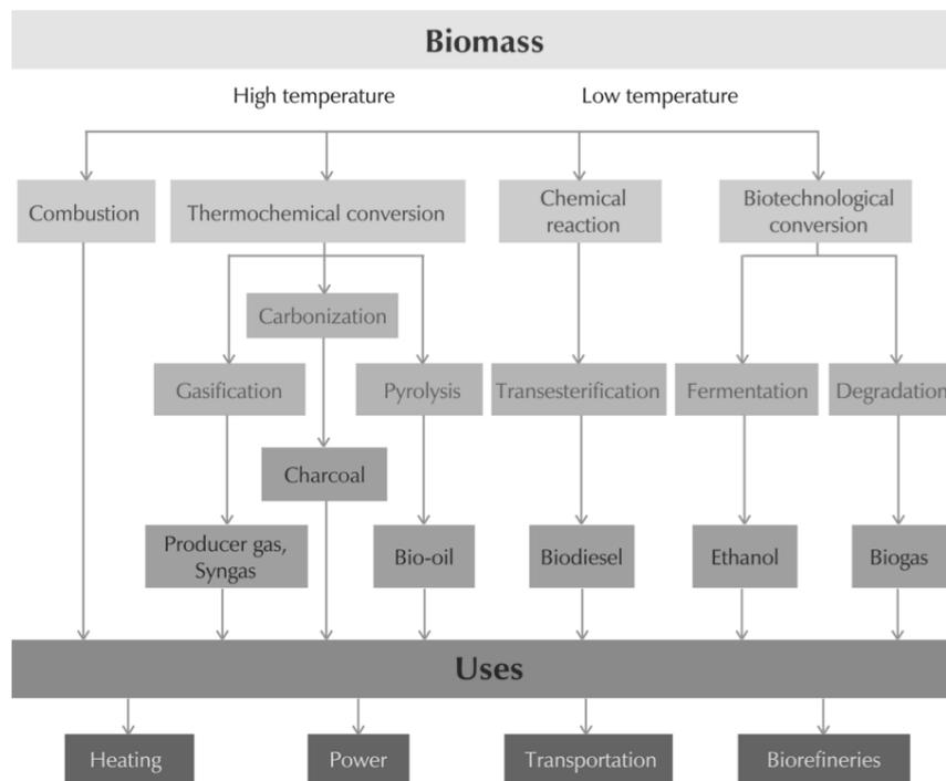
Figure 3.1. Main technology routes for bioenergy production. (ISPRES 2009)
